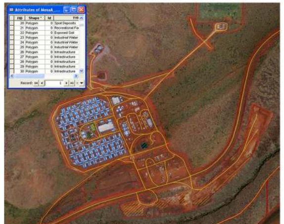
Mine Infrastructure Feature Detection and Attribution using Very High Resolution Satellite Imagery © DigitalGlobe (2011), Geoimage (2011)
